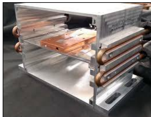
Figure 5.4: Example of The Test Bench Equipped with The Evaporator.
