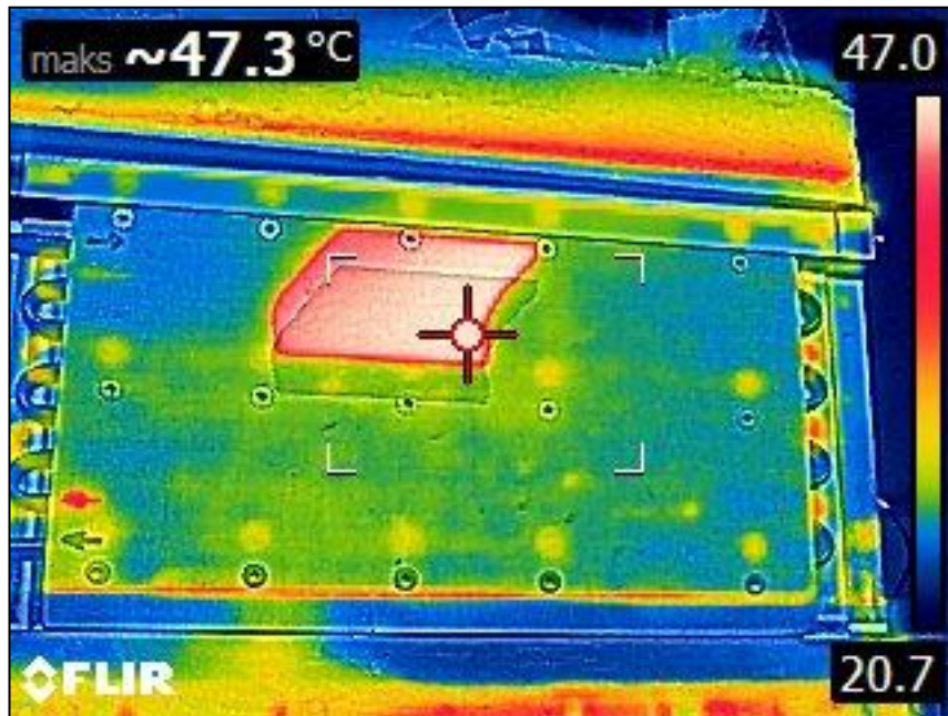
Figure 6.12: Evaporator Temperature Distribution at Full Load.
