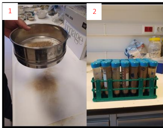
Figure 3.10: Laboratory analysis steps for soil texture analysis.
