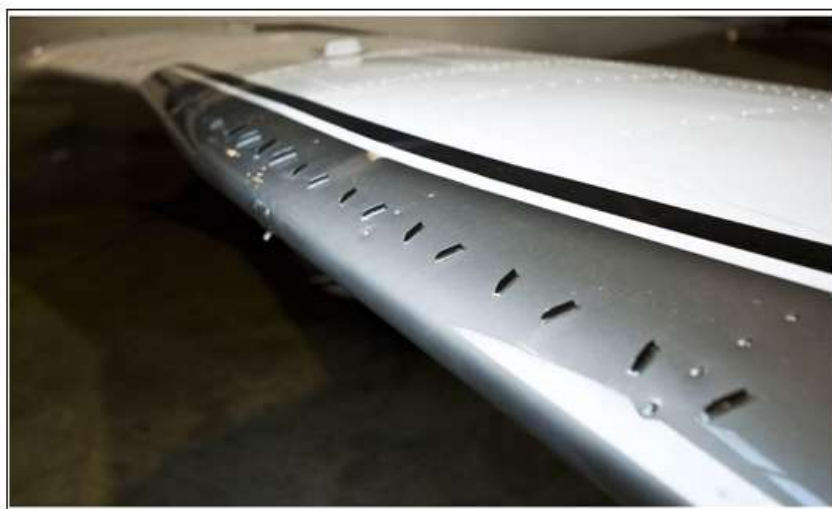
Figure 1.3: Counter-rotating vortex generators on an aircraft wing.
