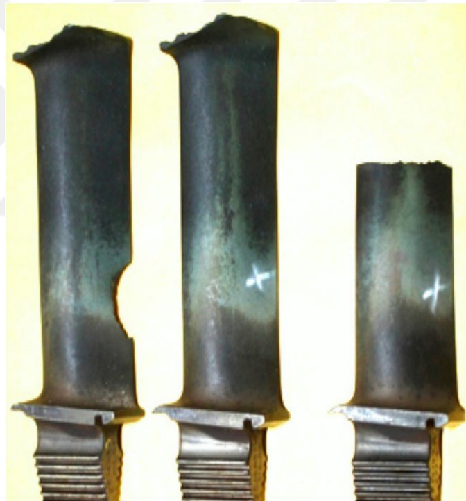
Figure 57. Fractured and Damaged Turbine Blade [24]
