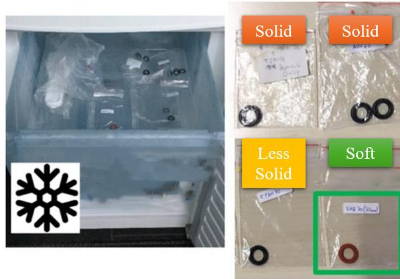
Figure 7.19: New O-Ring that maintains its flexibility under cold conditioning
