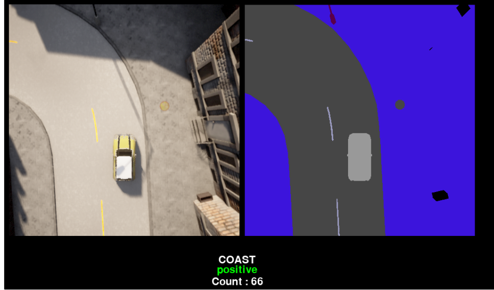
Figure 5.8: The human feedback collection user interface. The left image shows the top view of the car, the right image shows the semantic segmentation which is the model's observation. Current action, the feedback, and the feedback count are shown at the bottom of the interface. Feedback is provided through the keyboard by using the interface window.
