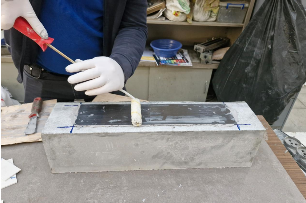
Figure 3.13: Ensuring full adhesion of the CFRP plate to the concrete.
