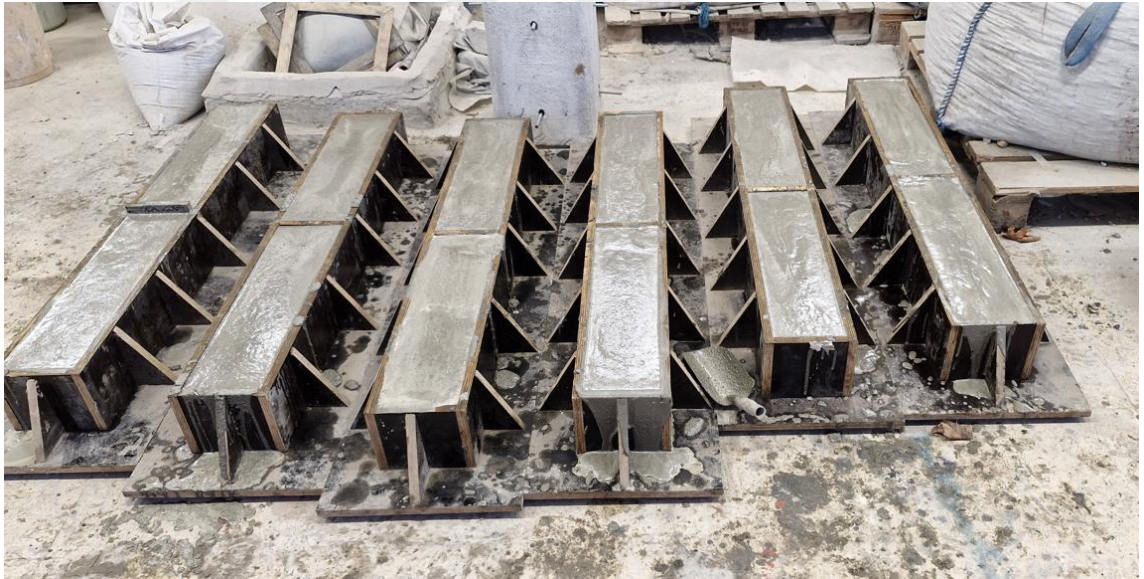
Figure 3.7: Samples placed in molds and kept for 24 hours.
