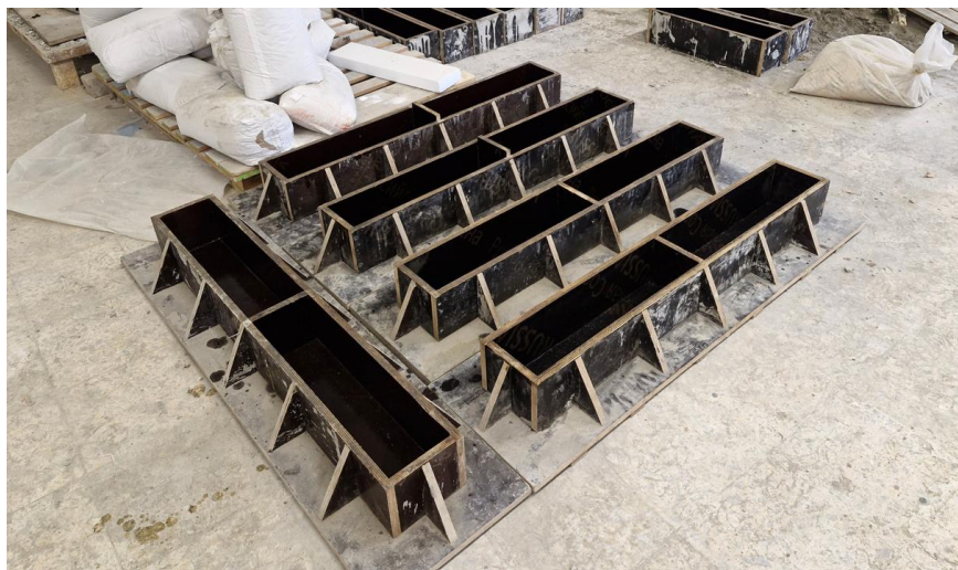
Figure 3.4: Sample Molds with Dimensions of 150x150x1220 mm.
