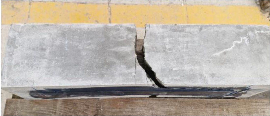
Figure 4.12: Fracture shape of beam sample and debonding of EP1.08-CNT0.5
