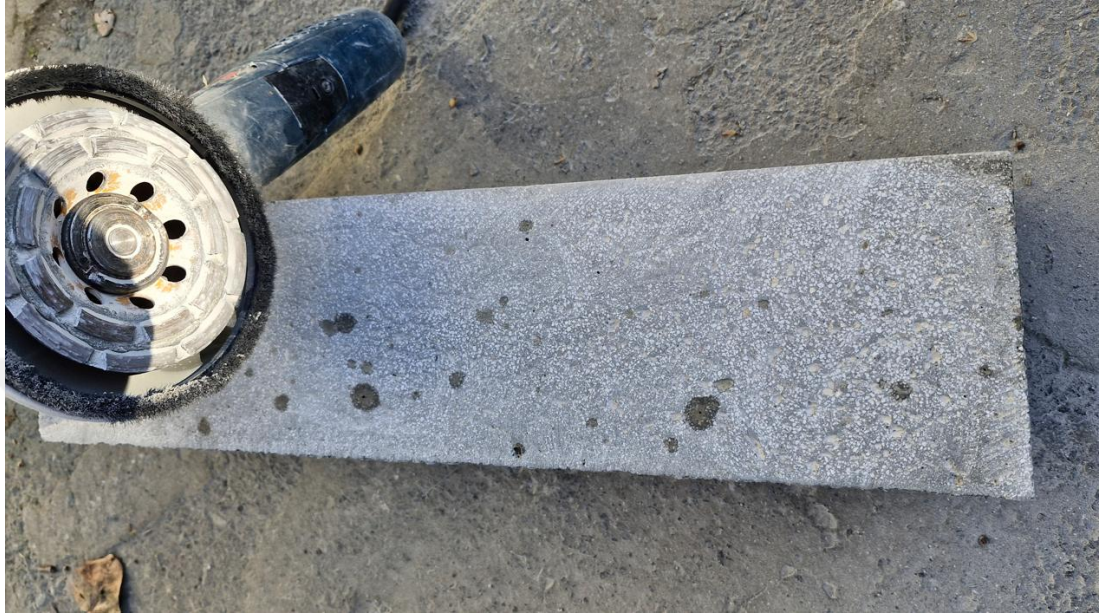
Figure 3.10: Beam sample surface after grinding.
