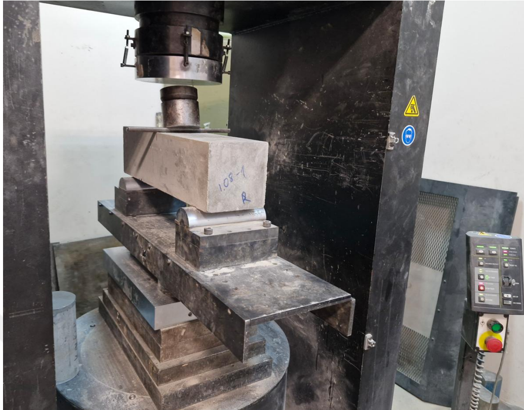
Figure 3.22. Placing the specimen in the equipment for the three-point bending test
