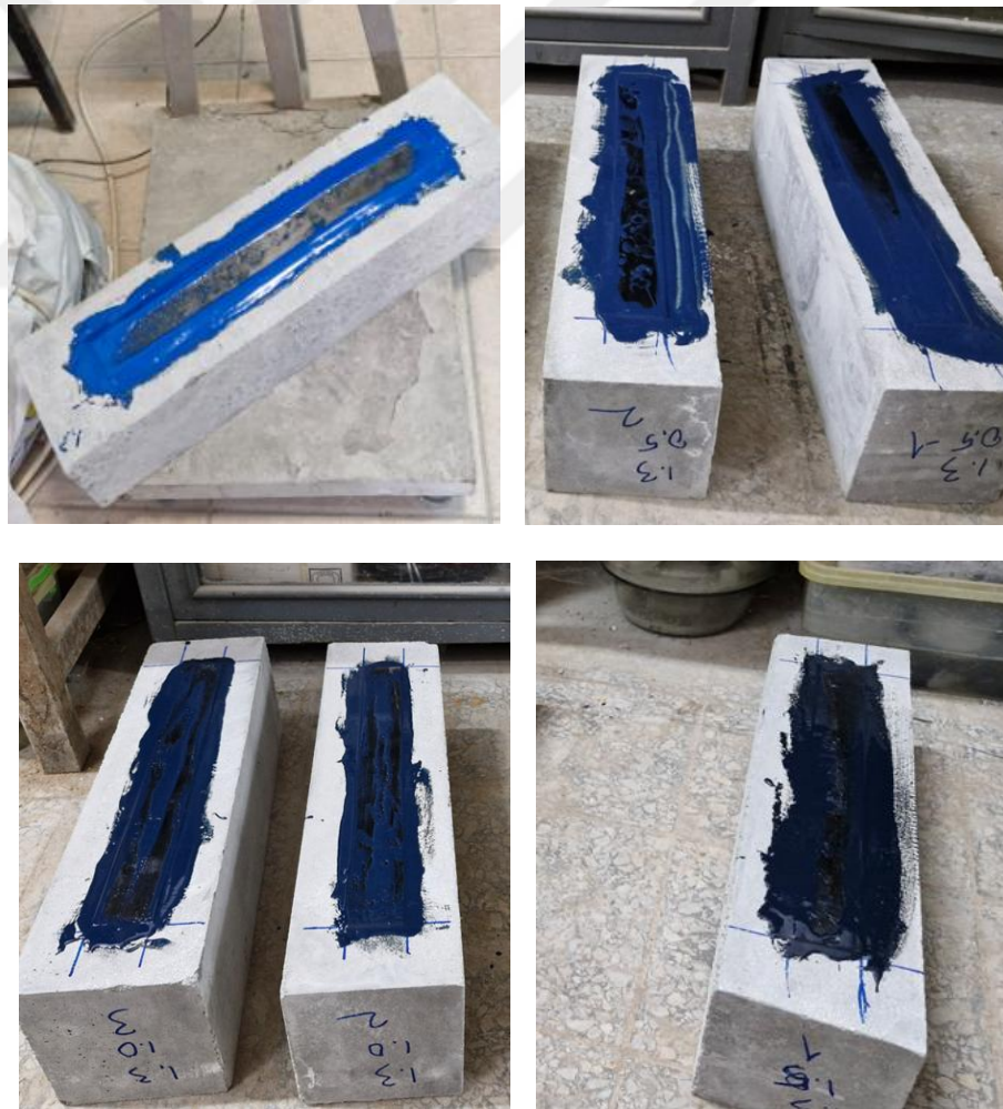
Figure 3.17: Samples produced with adhesive containing MWCNT (At top left; 0%, top right 0.5%, bottom left; 1.0%, bottom right; 1.5%, respectively.)
