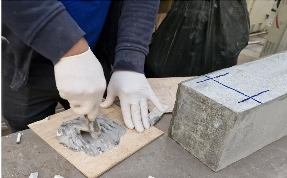
Figure 3.11: Preparation of epoxy-based adhesive before application.
