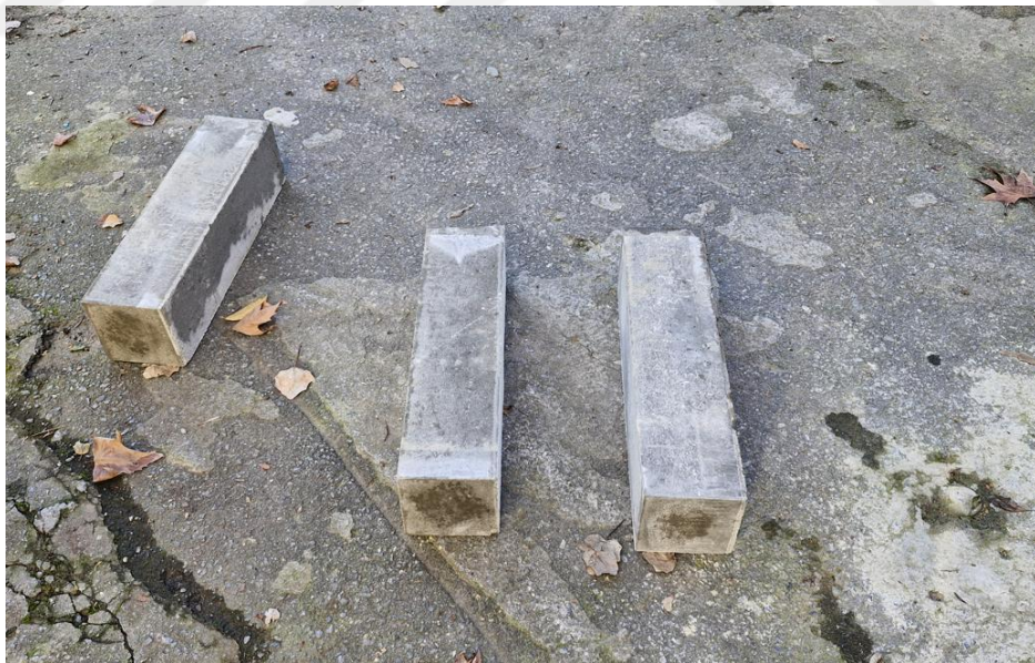
Figure 3.9: Samples removed from the cure pool on day 28.
