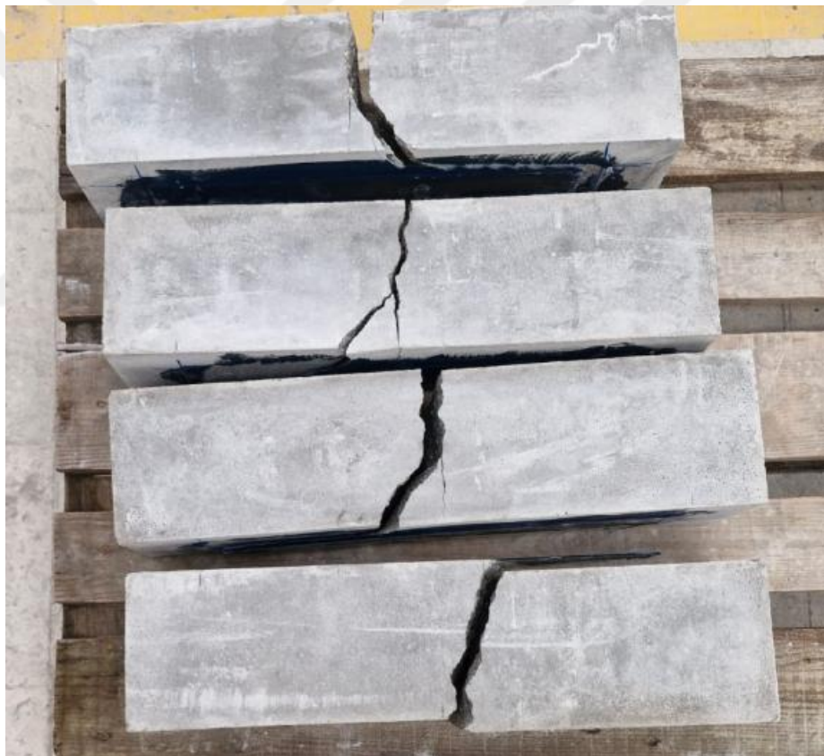
Figure 4.13: Fracture shape of beam samples with code EP-1.30
