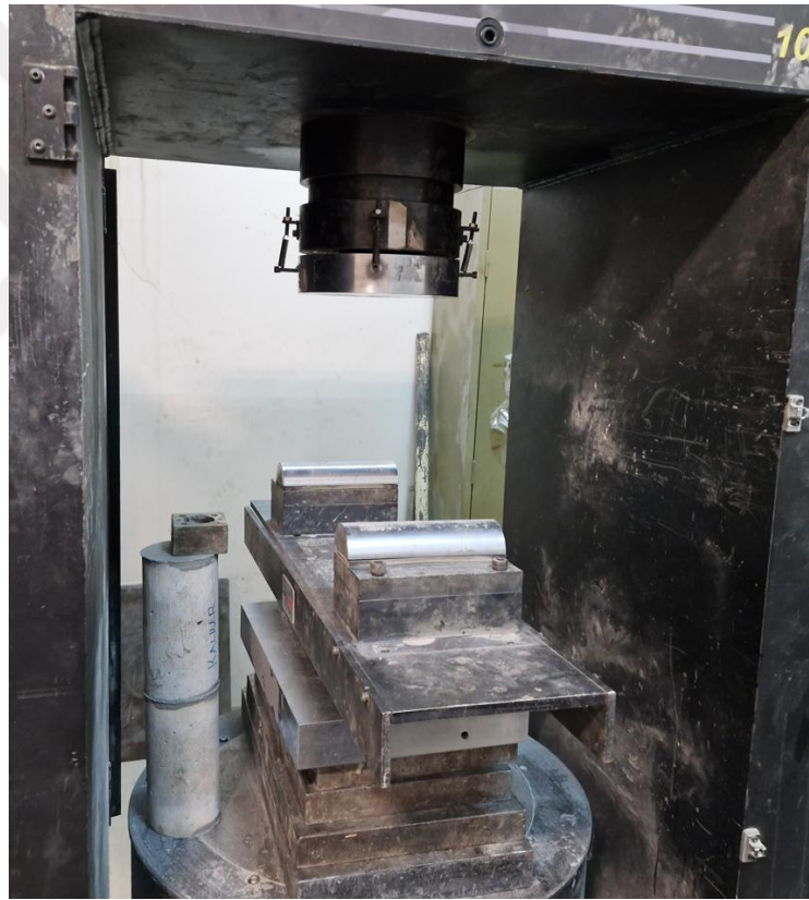
Figure 3.21. Three point bending test set up at Istanbul Technical University
