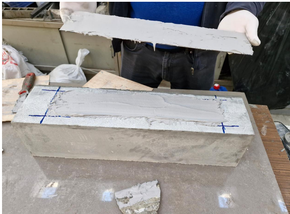
Figure 3.12: Applying the prepared resin homogeneously to both surfaces.
