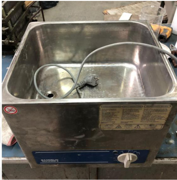
Figure 3.15: Sonicator used for mixing of MWCNT.
