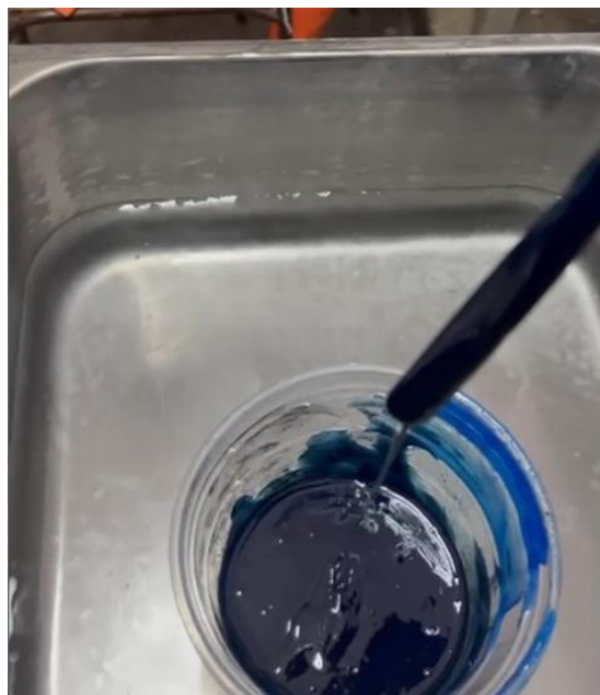
Figure 3.16: MWCNT-epoxy resin component A mixed in sonicator.
