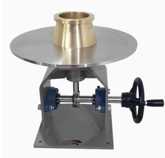
Figure 3.1: Cement spreading table according to TS EN 1015-3 [33].
