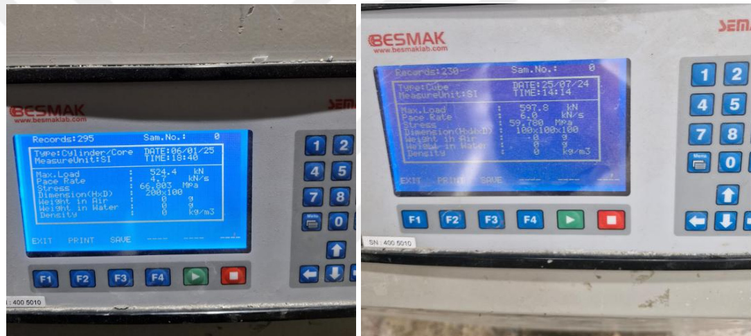
Figure 4.3. The compressive strength results of the hardened samples (On the left, the test result of the 28-day cylindrical sample with dimensions of 200x100 mm, on the right, the test result of the cubic sample with dimensions of 100x100x100 mm)
