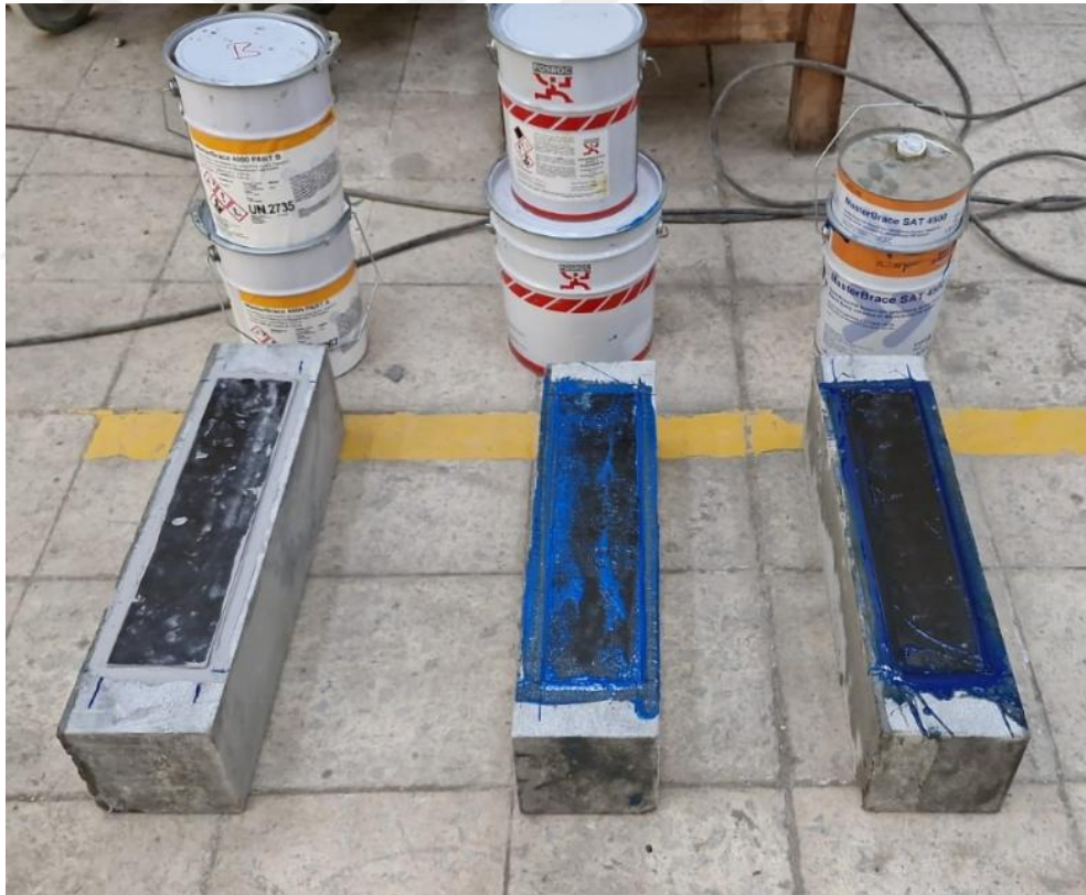
Figure 3.18: Beams produced during preliminary studies (with 100 mm wide CFRP plate and epoxy resin of 3 different densities)
