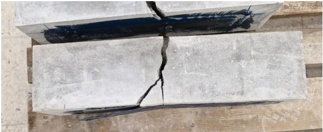
Figure 4.11: Fracture shape of beam sample and debonding of EP1.08-CNT0.5
