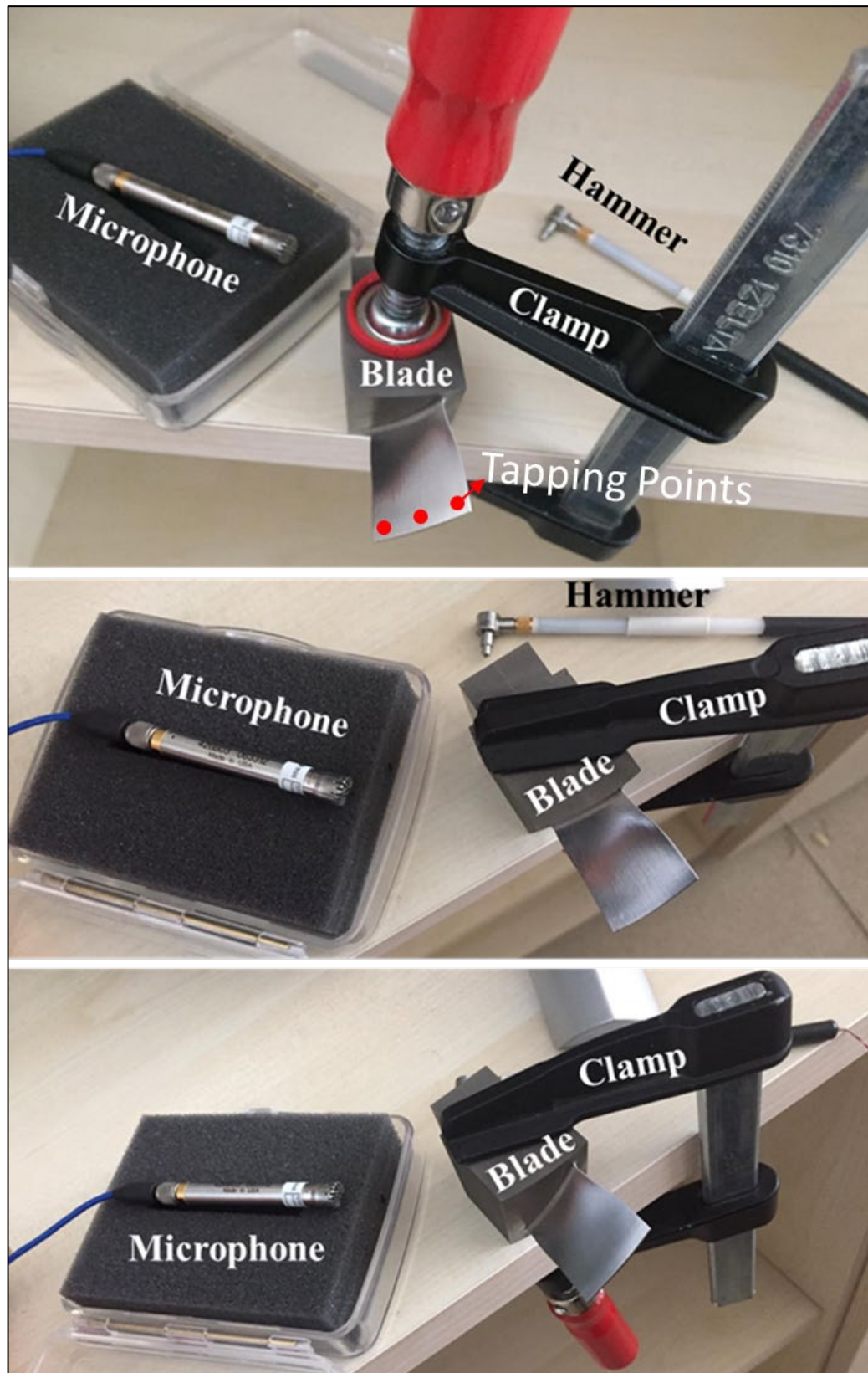
Figure 2.63: Test Setup with Microphone, Hammer, Clamp and Blade.
