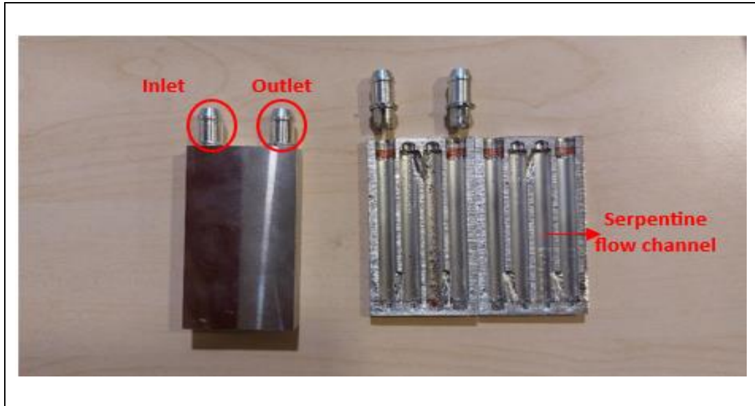
Figure 3.2: Aluminum cooling plate.
