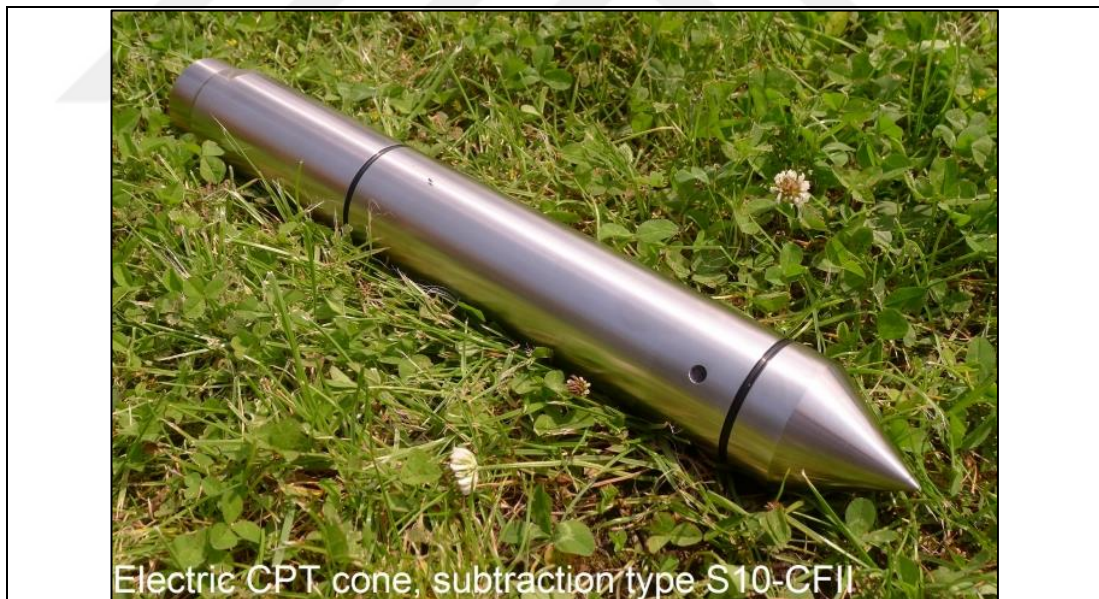
Figure 2.7: Electric piezometric cone penetrometer.
