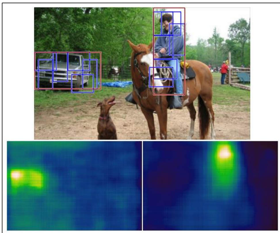
Figure 3.2: DPM samples on a car and a person model. Their corresponding appearance energy maps are given on the lower part.
