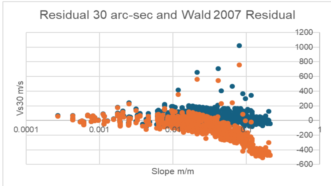
Figure 6.46: The residuals of the 30 arc-second slope gradient model compared to the residuals from the (Wald & Allen, 2007) study.
