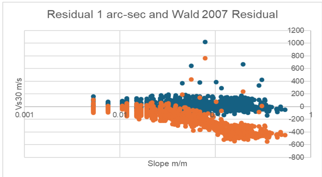
Figure 6.42: The residuals of the 1 arc-second slope gradient model compared to the residuals from the (Wald & Allen, 2007) study.
