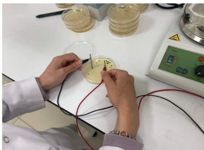
Figure 3.1: The application of DC electric current to the anode and cathode terminals for specified durations.
