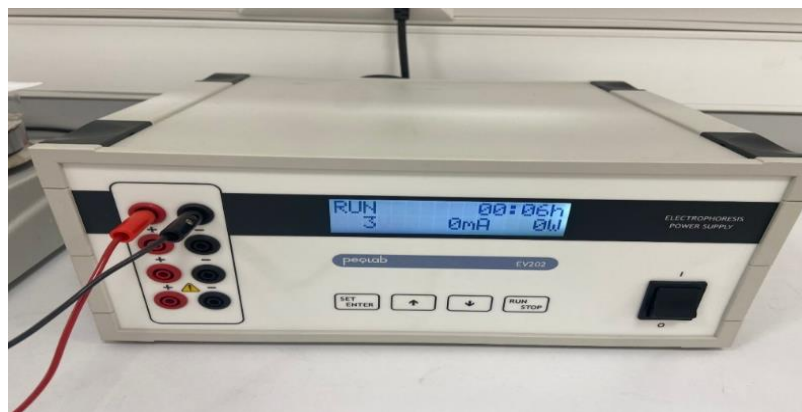
Figure 3.2: Device used for DC electric current peqlab EV202.
