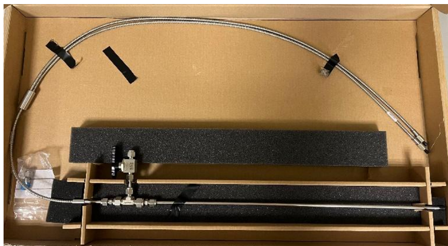
Figure 3.4: An optical fiber used as a measurement probe for high-temperature measurements at low pressures.
