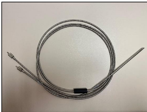
Figure 3.3: An optical fiber used as a reflection probe for powders and dense liquids.
