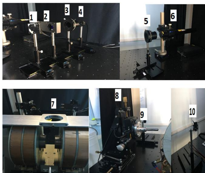
Figure 8.6: Component of MOKE device.
