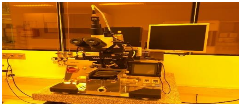
Figure 9.5: Mask aligner device was used for lithography.
