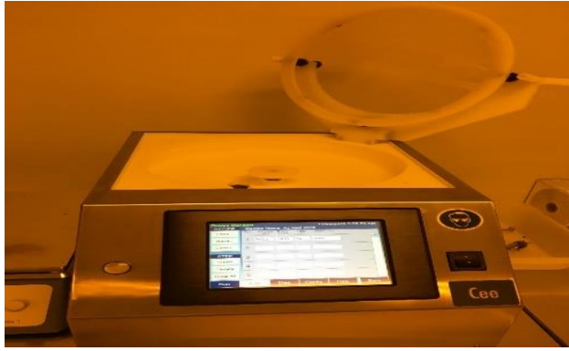
Figure 9.4: Spin coater was used for lithography.
