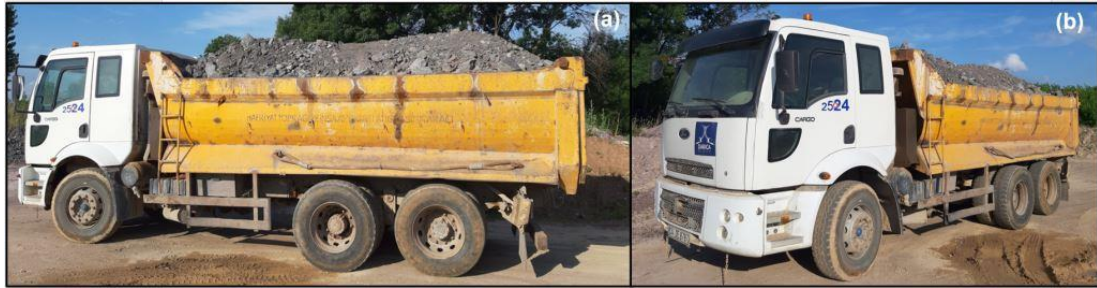
Figure 6.16: An actual 3 axle Ford Cargo 2524 model truck for loading of APT test.
