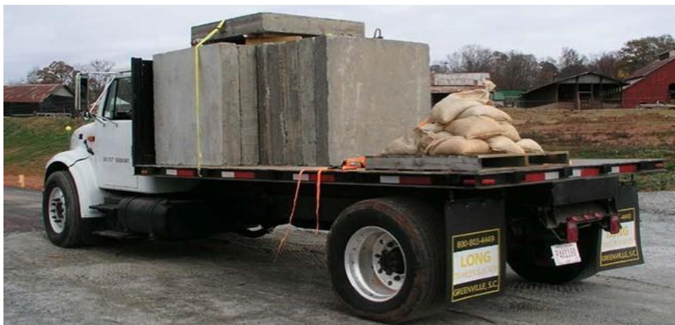
Figure 2.23: Conventional 2-axle truck with each axle modified to apply a load of 80 kN [Valero et al., 2014].
