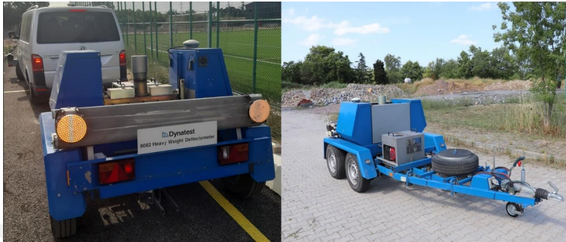
Figure 2.15: Dynatest 8082 deflectometer with 320 kN capacity used in this study.
