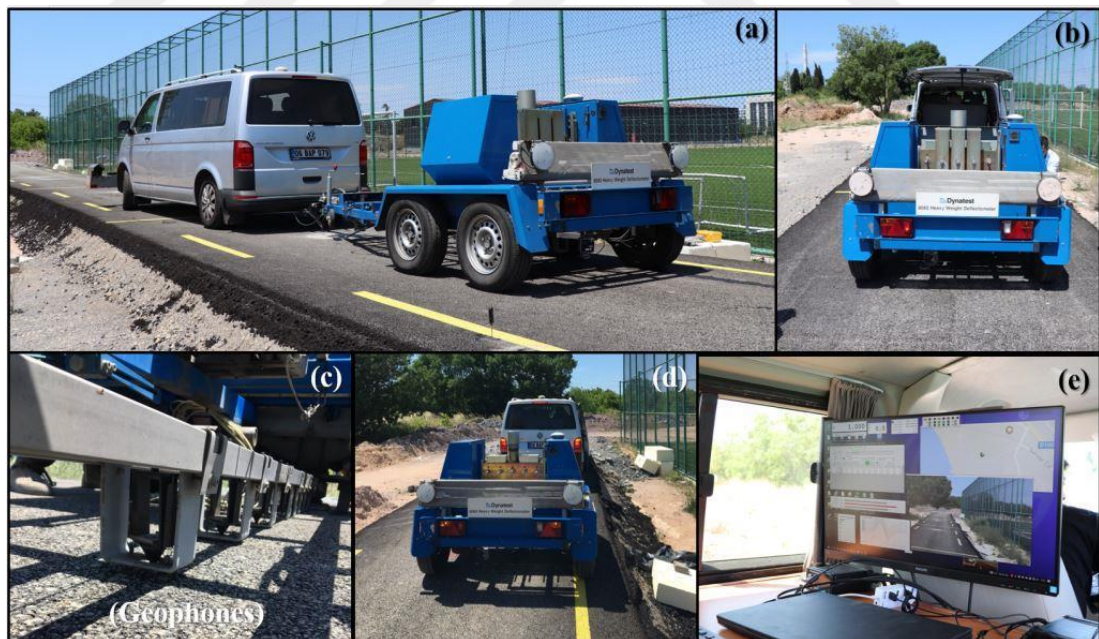
Figure 6.24: Falling weight deflectometer (FWD), a-b) Setup of FWD equipment, c) Geophones, d-e) Applying the load and recording the load-displacement curves with the software.
