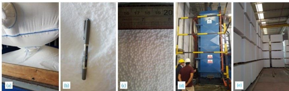
Figure 2.1: Production stages: a-b) Raw polystyrene, c) Pre-expansion, d) Molding, e) Resting for dimensional stability in the stock area of the molding facility [  zer, 2021].
