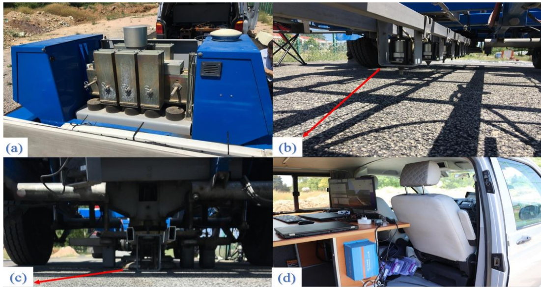
Figure 2.16: FWD set-up: a) Loading system with weights, b) Geophones, c) Loading plate, d) Data logger and computer.
