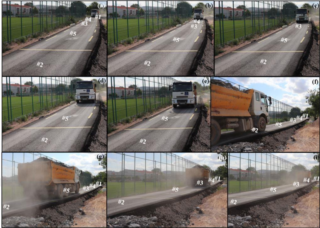
Figure 6.17: Accelerated pavement test a-e) Loading in east-west direction, f-i) Loading in west-east direction.
