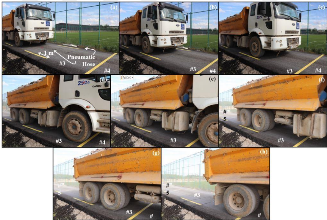
Figure 6.18: Truck passage through pneumatic hoses during accelerated pavement test, a-h) Loading in east-west direction.
