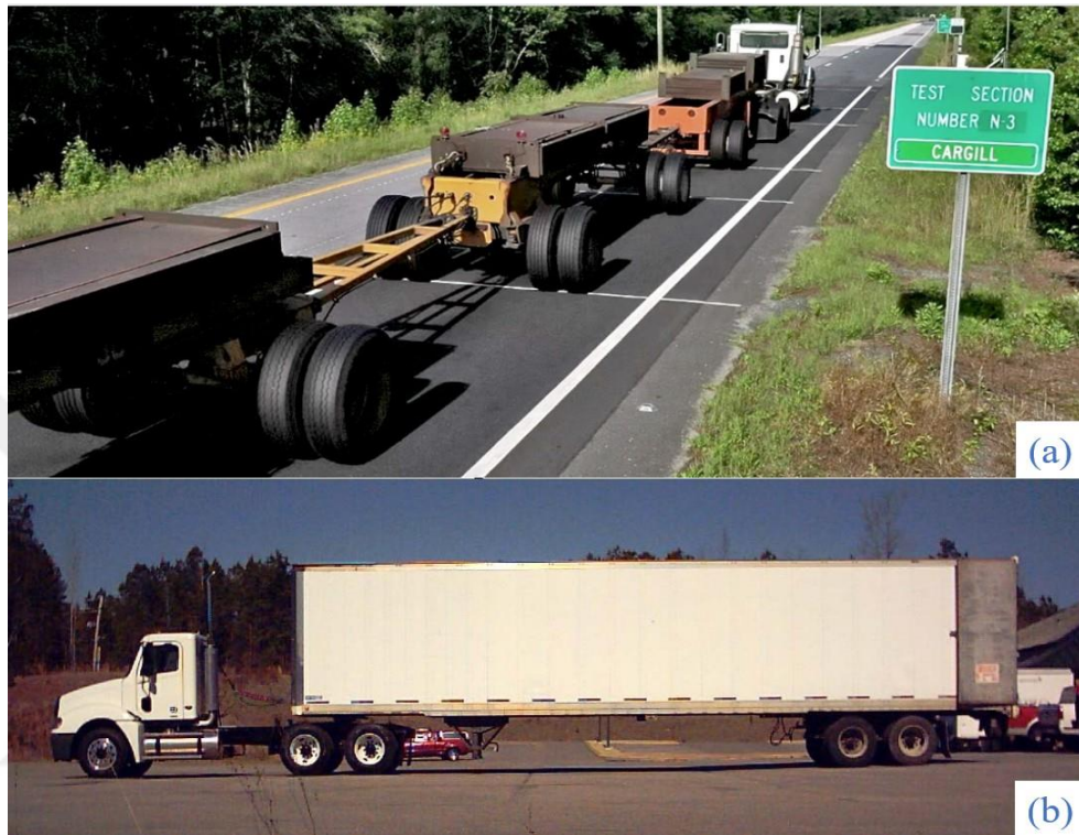
Figure 2.22: NCAT APT actual vehicles, a) Triple trailer [Web 2, 2023], b) Box trailer [Timm and Priest, 2005].
