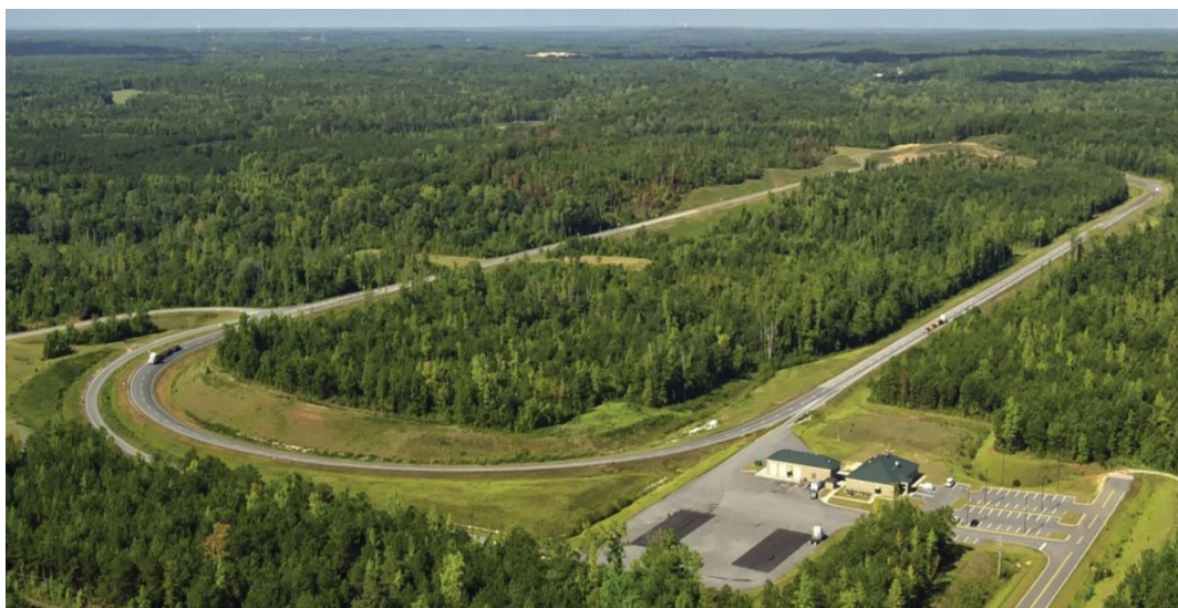
Figure 2.21: The full-scale APT track for innovation and research of pavement technologies in the US National Center for Asphalt Technology [Web 1, 2023].
