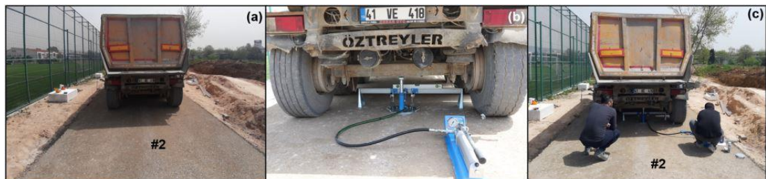
Figure 6.4: PLT, a) A truck loaded to its capacity pulls up to the test location in the Configuration #2, b) Installation of PLT setup, c) Performing the PLT according to the defined loading and unloading protocol.
