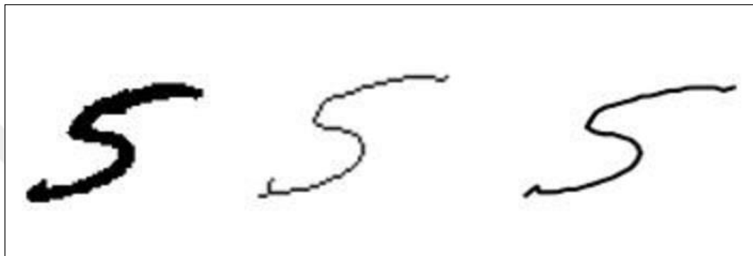
Figure 3.1: From left to right; the spline curve created with the raw handwritten character, the skeleton image of the character, and the control points.
