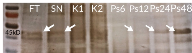
Figure 4.3: Silver staining analysis of purified CtFDH at 25 °C, pH 6.0 with casamino acids; FT: Flowthrough; SN: Supernatant; K1: Control supernatant wild type X33; K2: Control supernatant samples from P. pastoris containing laccase gene; Ps6: Purified sample at 6 h; Ps12: Purified sample at 12 h; Ps24: Purified sample at 24 h. Ps48: Purified sample at 48 h.
