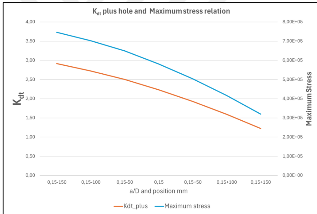
Figure 2.162: K dt values and Maximum stress for plus hole change position
