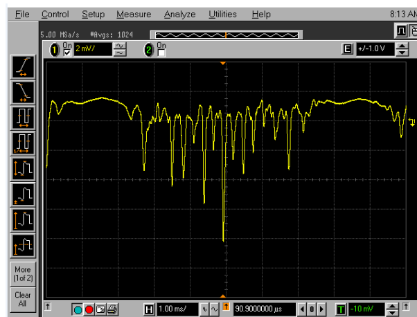
Figure 5.12: 15 Zeeman resonance of the DROR signal for 6S_{1/2} (F=3) \leftrightarrow 6S_{1/2} (F=4) transition at 12,2 mW fixed laser power and 500 V/m electric field strength.
