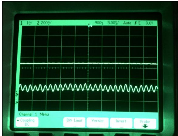
Figure 4.7: The Doppler signal (top) locked on the 6S_{1/2}(F=4) - 6P_{3/2}(F=4) transition that does not change with time, on Cs1 reference tube and the reversed error signal (bottom).
