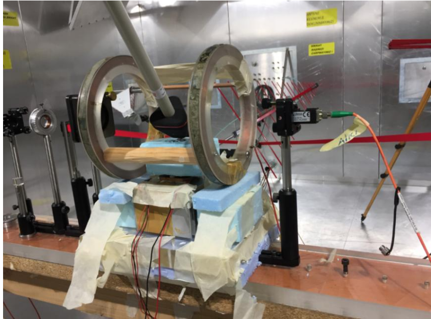
Figure 5.8: Electric field probe at the point of Cs2 test tube in Helmholtz coil.
