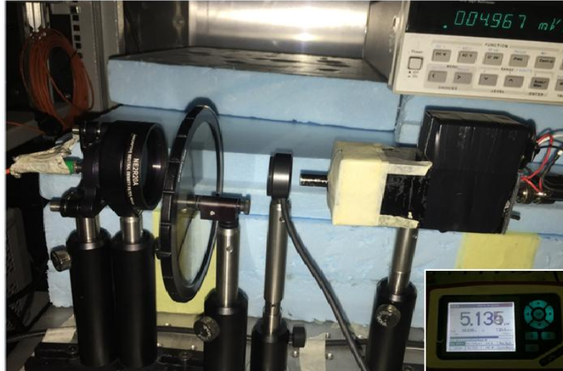
Figure 5.4: Photo from the photodiode linearity measurement setup.
