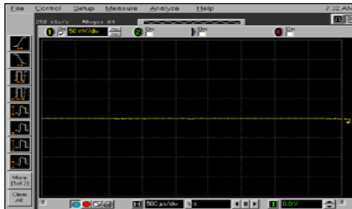
Figure 4.8: The Doppler signal locked on 6S_{1/2}(F=4) - 6P_{3/2}(F=4) transition that does not change with time, on Cs2 reference tube.
