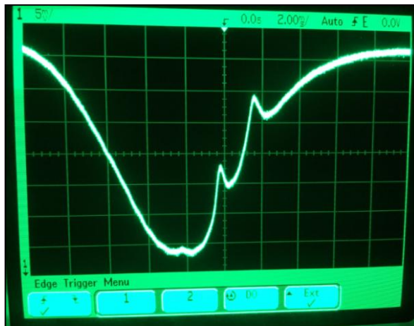
Figure 4.5: Sub-Doppler resonances in reference Cs1 tube displayed on oscilloscope.
