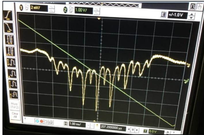
Figure 4.12: Zeeman sublevels of the DROR resonance on oscilloscope display.
