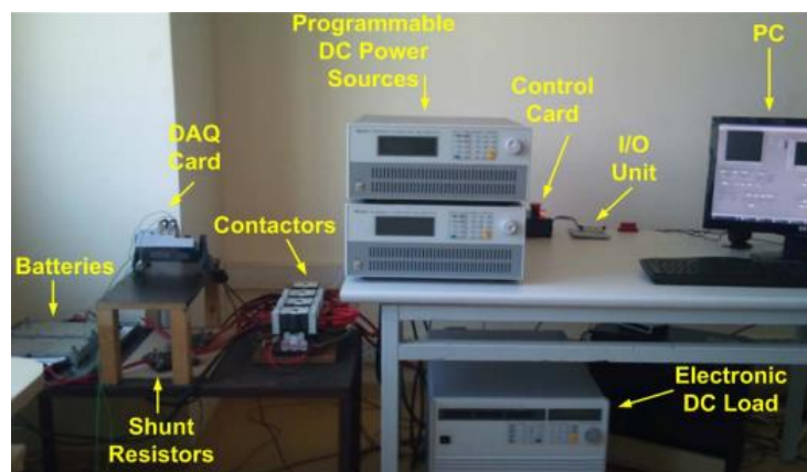
Figure 3.3: Experimental setup photograph.
