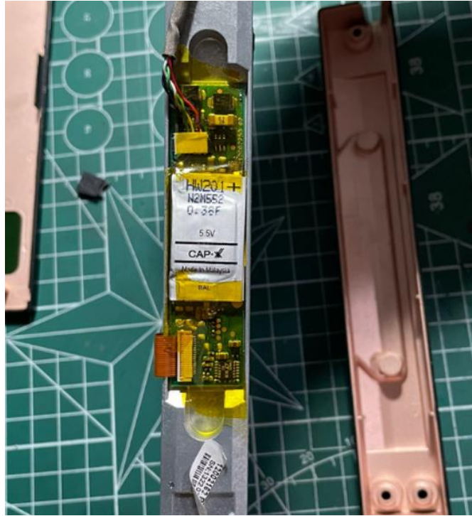
Figure A.2: Tobii X2-30 with replaced capacitor.
