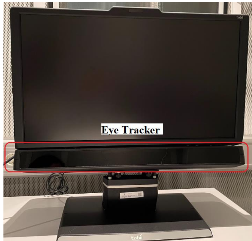
Figure 1.4: Tobii TX300 eye tracker device with removable 23” monitor.
