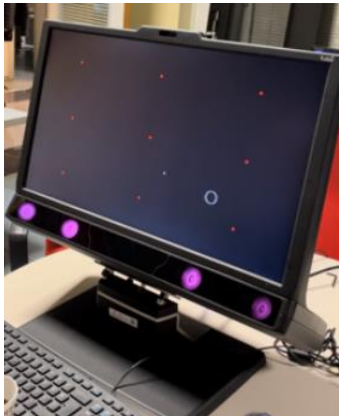
Figure A.3: Calibration issue for Tobii TX300 device.
