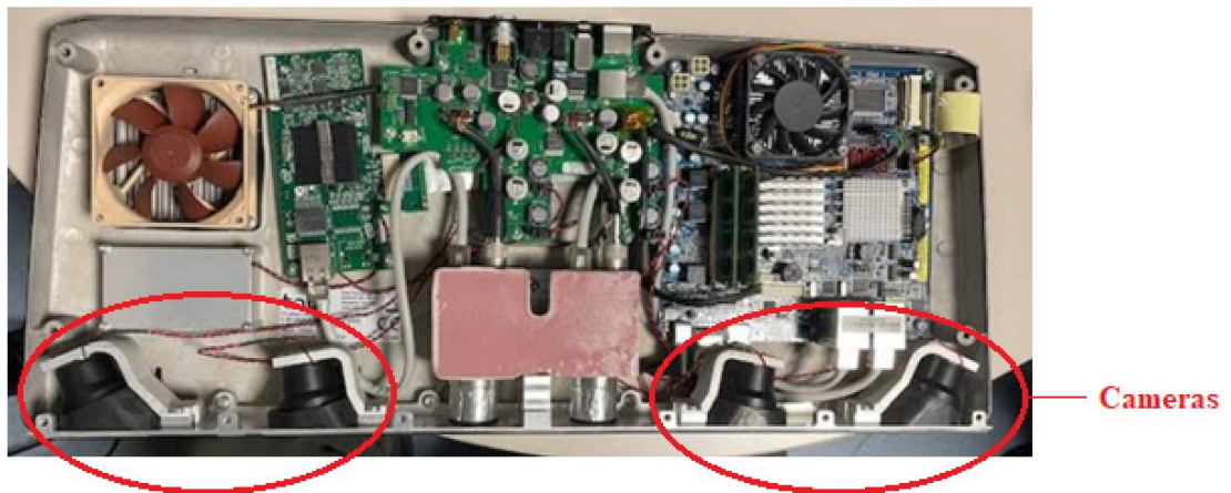
Figure A.4: Casing opened for Tobii TX300 device
