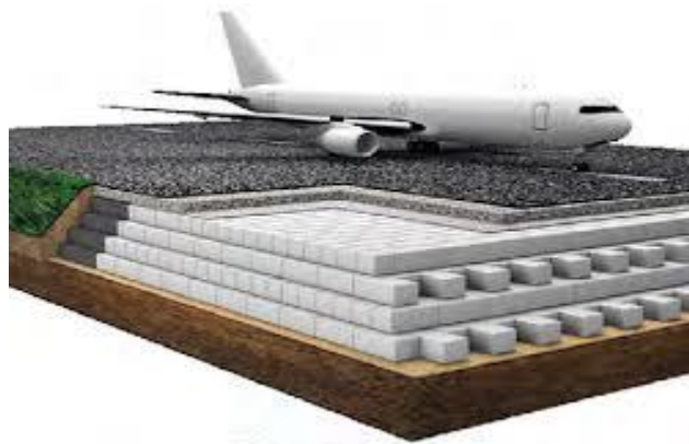
Figure 2.16: Conceptual geofoam block placement in an airport (Tolga, 2020).
