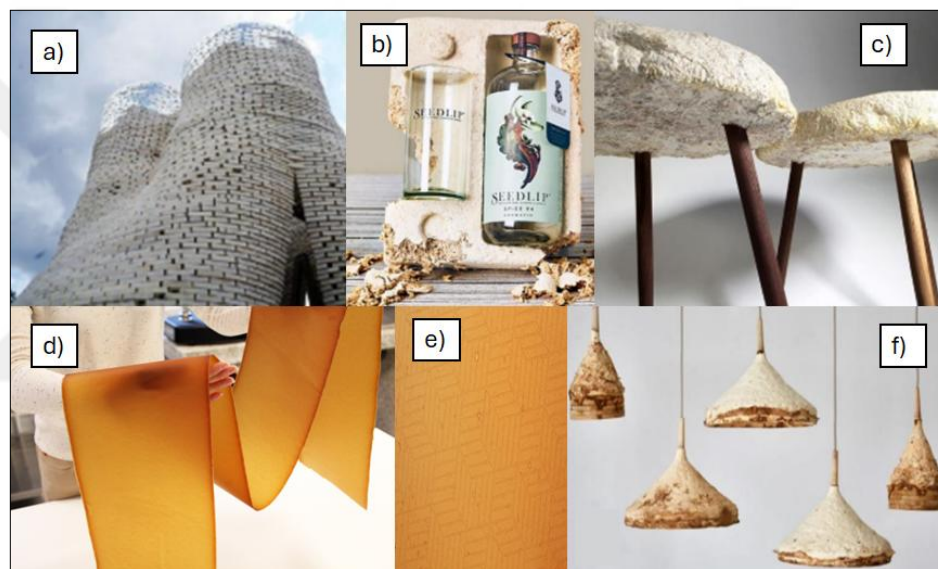
Figure 1.18: Some applications of mycelium biocomposites. In a) insulation, b) packaging, c) furniture, d) vegan artificial leather, (e) the pattern of this leather) f) lighting. Adapted from: [45], [48].
