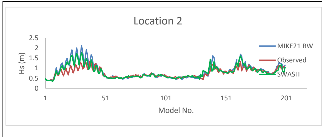
Figure 5.2: Comparison MIKE21 BW and SWASH default models with observed H_s in location 2.
