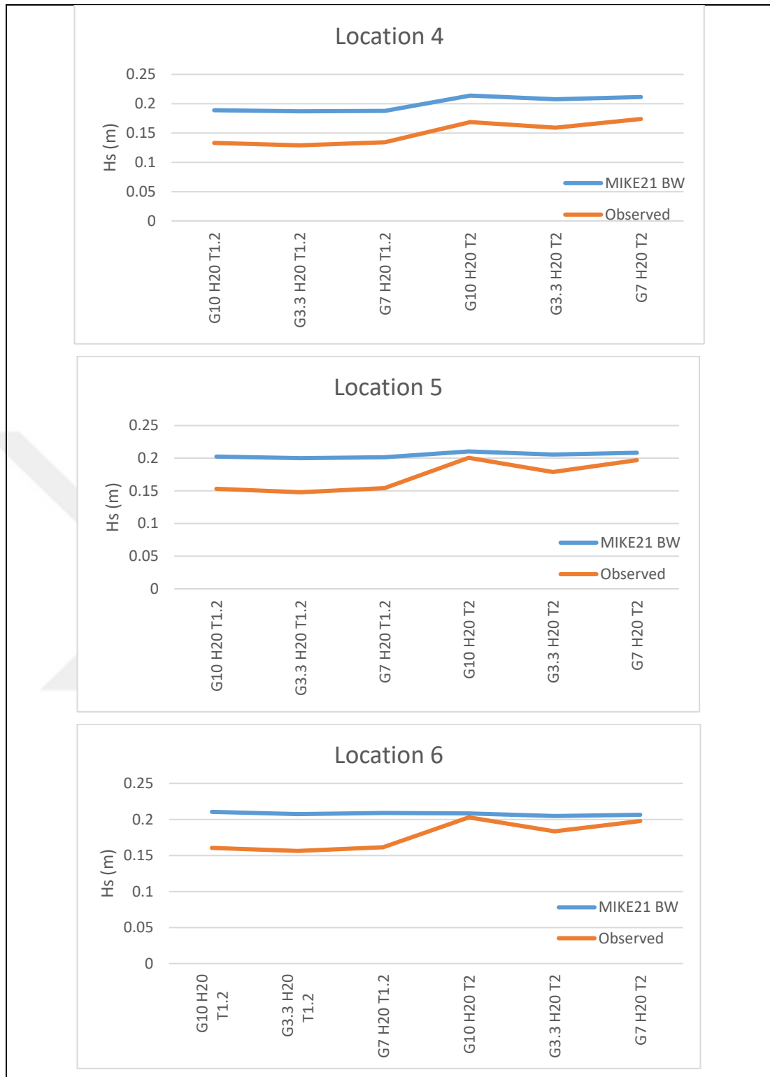
Figure 4.9: Comparison of JONSWAP spectrum H_s of 3 locations in the deepest water in default MIKE21 BW model and observed H_s .
