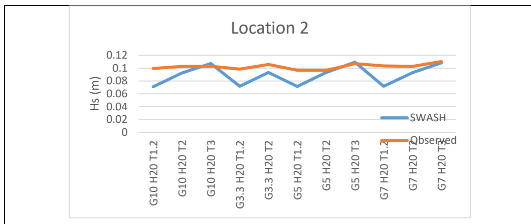
Figure 4.11: Comparison of H_s of location 2 in the shallowest water in default SWASH model with observed.
