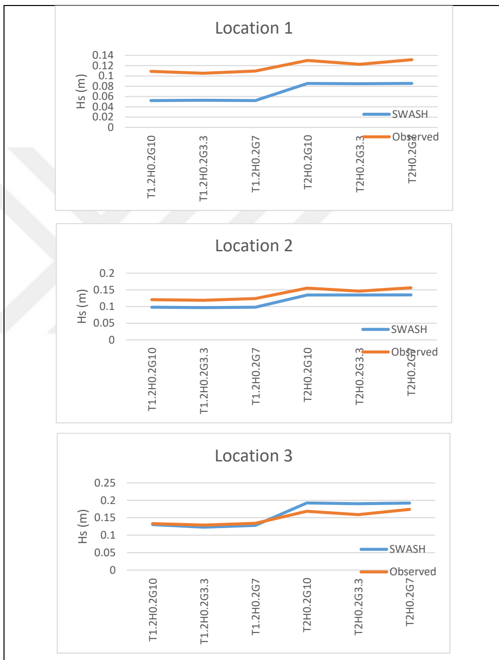
Figure 4.13: Comparison of H_s of 3 locations in the shallowest water in default SWASH model with observed.
