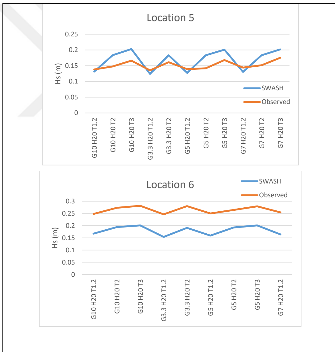
Figure 4.12: Comparison of H_s of 2 locations in the deepest water as time-series in default SWASH model with observed.
