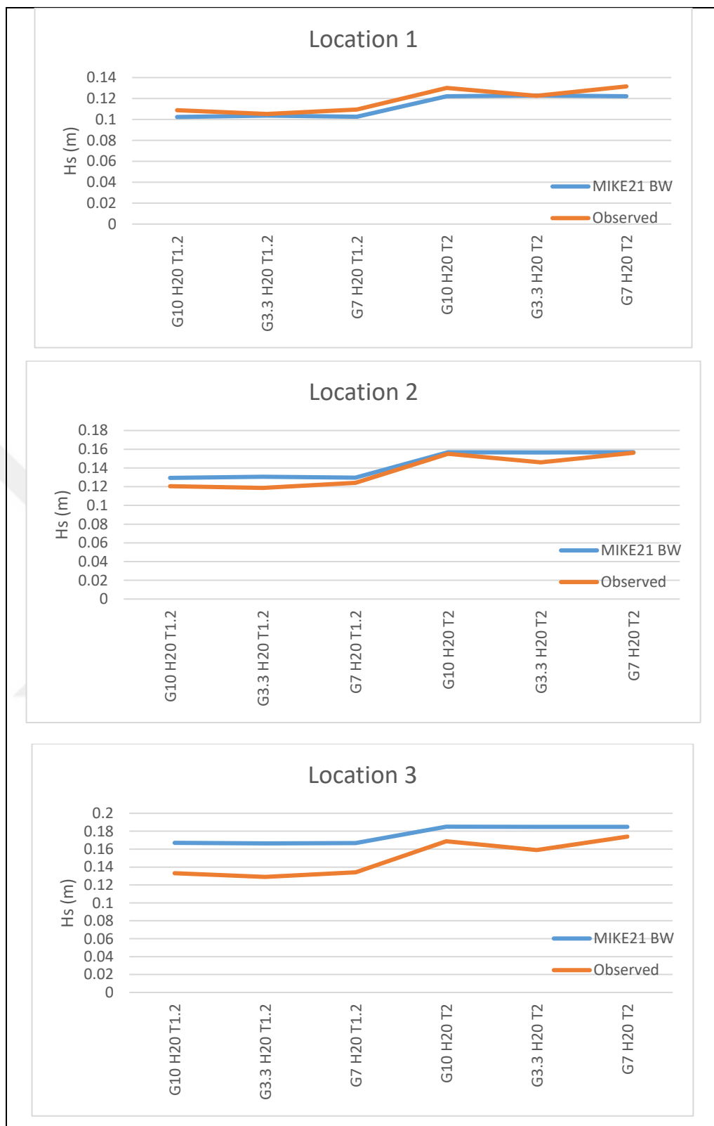
Figure 4.8: Comparison of JONSWAP spectrum H_s of 3 locations in the shallowest water in default MIKE21 BW model and observed H_s .
