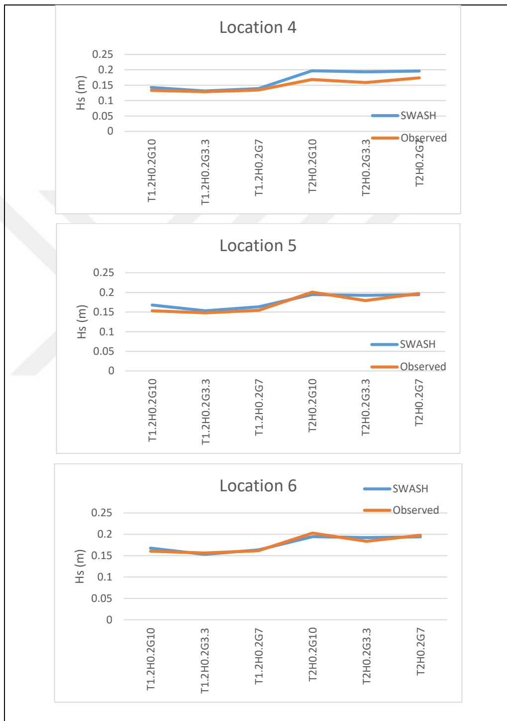
Figure 4.14: Comparison of H_s of 3 locations in the deepest water in default SWASH model with observed.
