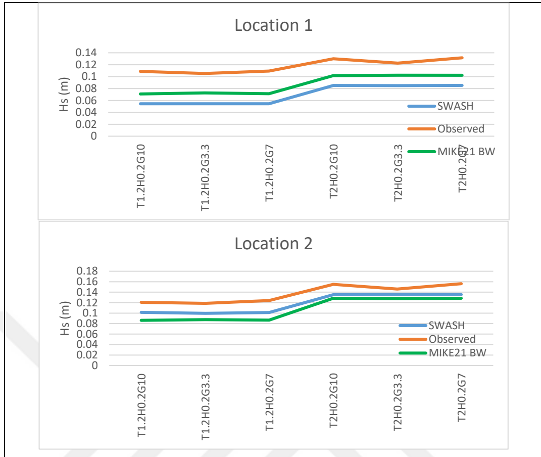
Figure 5.8: Comparison H_s values from experimental observation, MIKE21 BW and SWASH calibrated JONSWAP model in location 1, 2.
