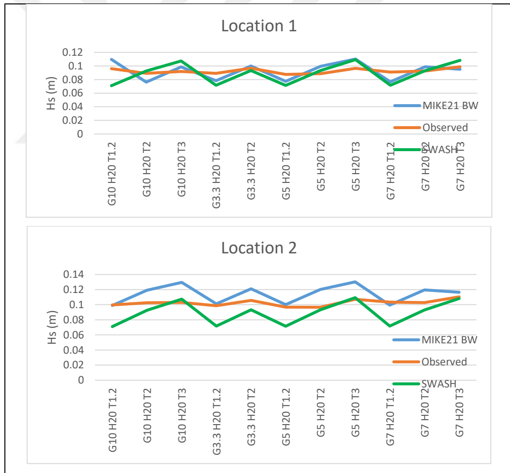
Figure 5.5: Comparison H_s values from experimental observation, MIKE21 BW and SWASH default JONSWAP model in location 1, 2.
