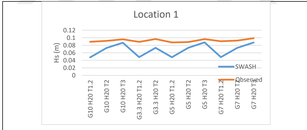
Figure 4.10: Comparison of H_s of location 1 in the shallowest water in default SWASH model with observed.
